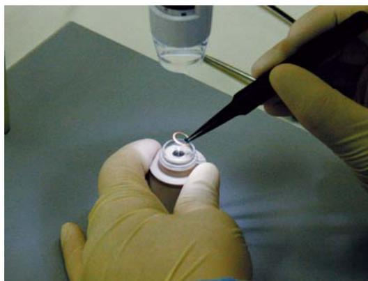
**Tensometer being placed on a soft contact lens. The tensometer is non-invasive and does not affect the person's vision. The sensor measures intraocular pressure around the clock.**
